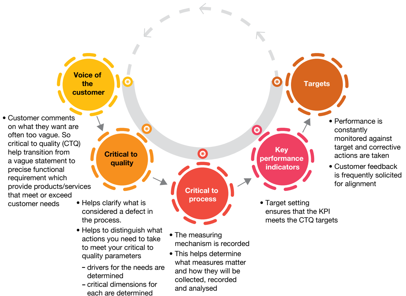
Figure 3: Measuring what matters starts with understanding customer requirements and converting them to critical to quality (CTQ) parameters
